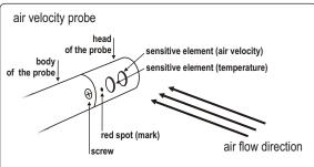
The red point on the probe's head is a mark that must be placed face to the airflow. Then, the probe is perpendicular to the airflow.
